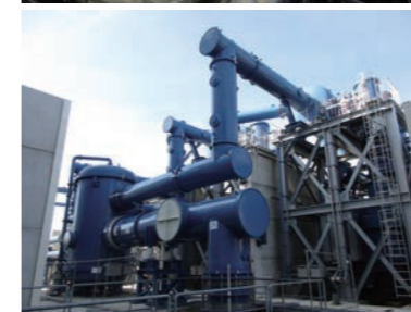
Nuclear fusion experimental equipment (Top: Inside of the plasma vacuum vessel (Photos courtesy of National Institute for Fusion Science)/Bottom: Power test equipment for neutral beam injector for ITER)
