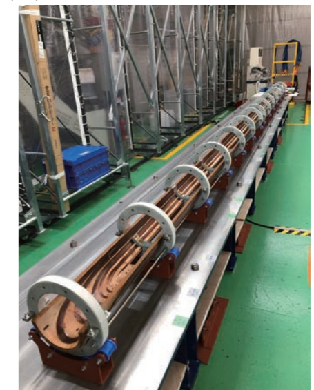
Accelerator for research (Superconducting magnets for the High Luminosity LHC Upgrade of CERN (Total length: 7m))
