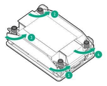
7. Set the anti-tilt wires to the unlocked position.
