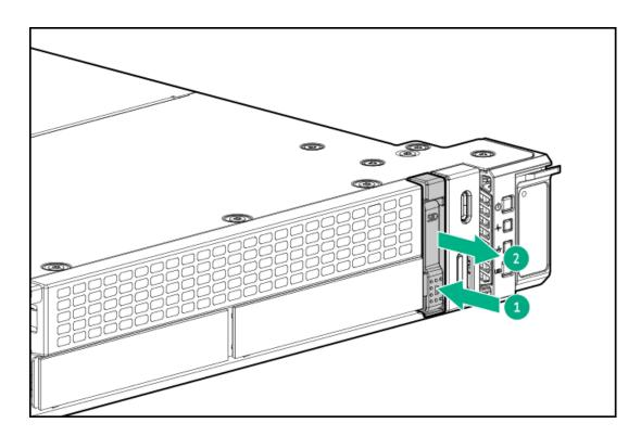
2. After the display ejects, rotate the display to view the LEDs.
