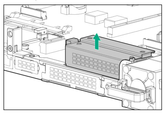
10. Using a T-15 Torx screwdriver, remove the rear riser support bracket.
