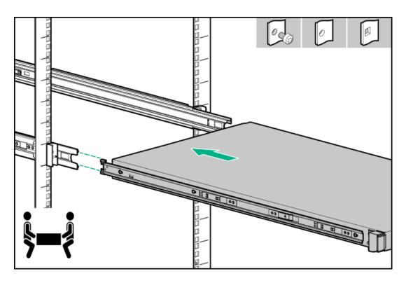
2. Open the chassis ears, and then tighten the shipping screws.
