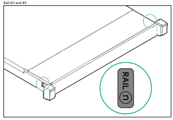
Rail identifier stamps on the inner rail of the friction rack rail
