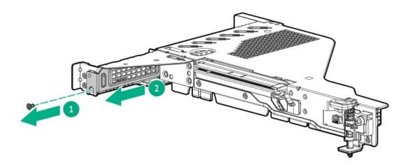
9. Use a T-10 Torx screwdriver to Install the expansion board.
