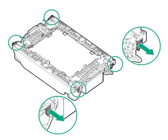
d. Lift the processor carrier away from the heatsink.
