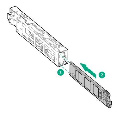
8. Slide the carrier inside the boot device cage and push the button. There will be an audible click when the latch locks into place. Ensure that the latch is fully engaged.
