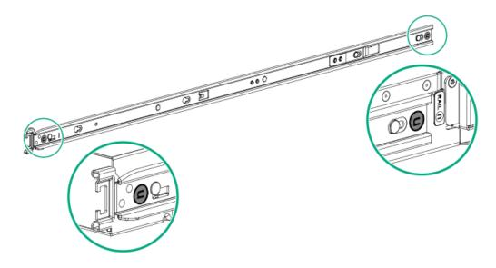
Rail identifier stamps on the mounting rail of the friction rack rail
