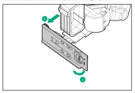
3. Install the CMA brackets to the inner and outer rails.
