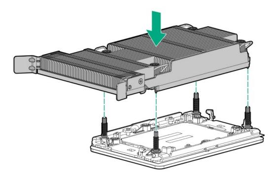
d. Set the anti-tilt wires to the locked position.
