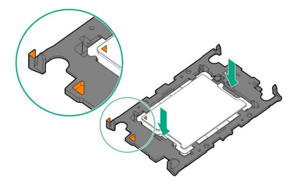
b. Verify that the processor is properly latched on the processor carrier.
