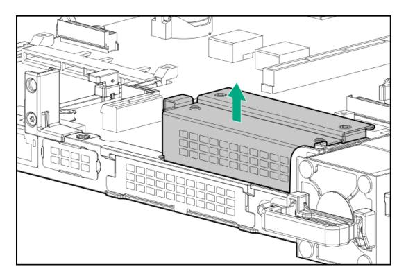
8. Install the secondary riser cage.
