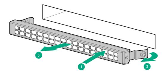
8. Install the optical drive bracket.
