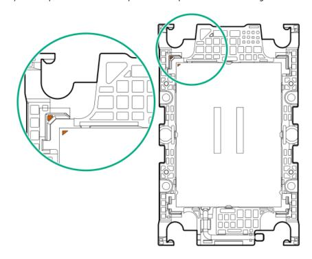
c. Verity that the processor is properly secured by the carrier snaps.
