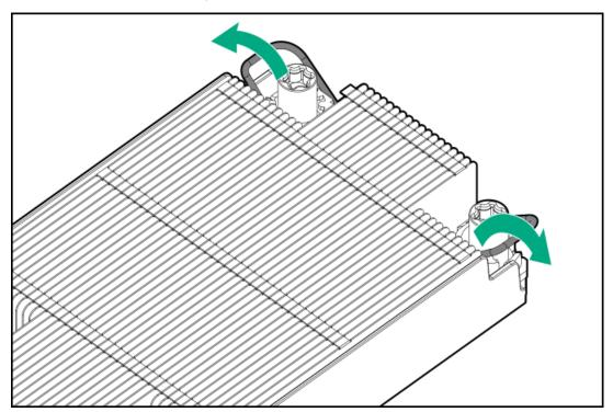
e. Tighten one pair of diagonally opposite heatsink screws, and then tighten the other pair of heatsink screws.
