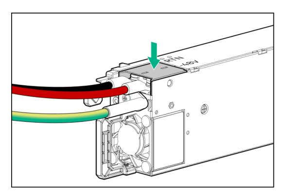
7. Secure the ground, positive return, and negative input wires in the strain relief strap.
