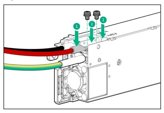
6. Install the protective cover on the DC power supply.
