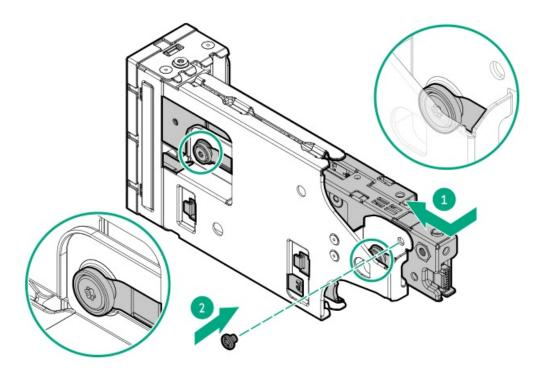
9. Install the boot device bracket into the multipurpose cage.
