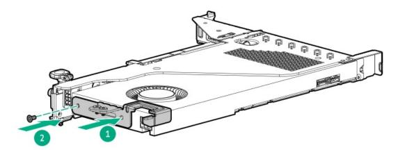
8. Install the GPU in the riser cage.
