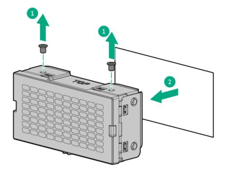
• If a drive cage is installed in Box 5, remove the drive cage.
