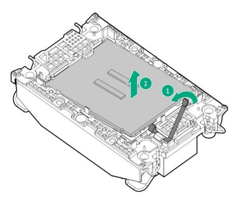
c. Starting from the pin 1 corner and moving in an opposite manner, disengage the processor carrier release tabs from the heatsink.
