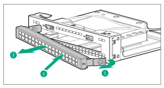
2. Install the optical drive bracket.
